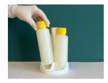
Align the round recesses in the lid with the caps and filters of the CellScrew® minis.
