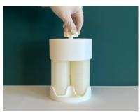
The CellScrew® mini TriDock is operated similarly to a CellScrew® 6K or 10K, by placing it on an angled (10 ° - 15 °) roller device. The CellScrew® mini TriDock must rotate clockwise when observed from above, with a rotational speed ranging from 0.2 to 2 rpm.
